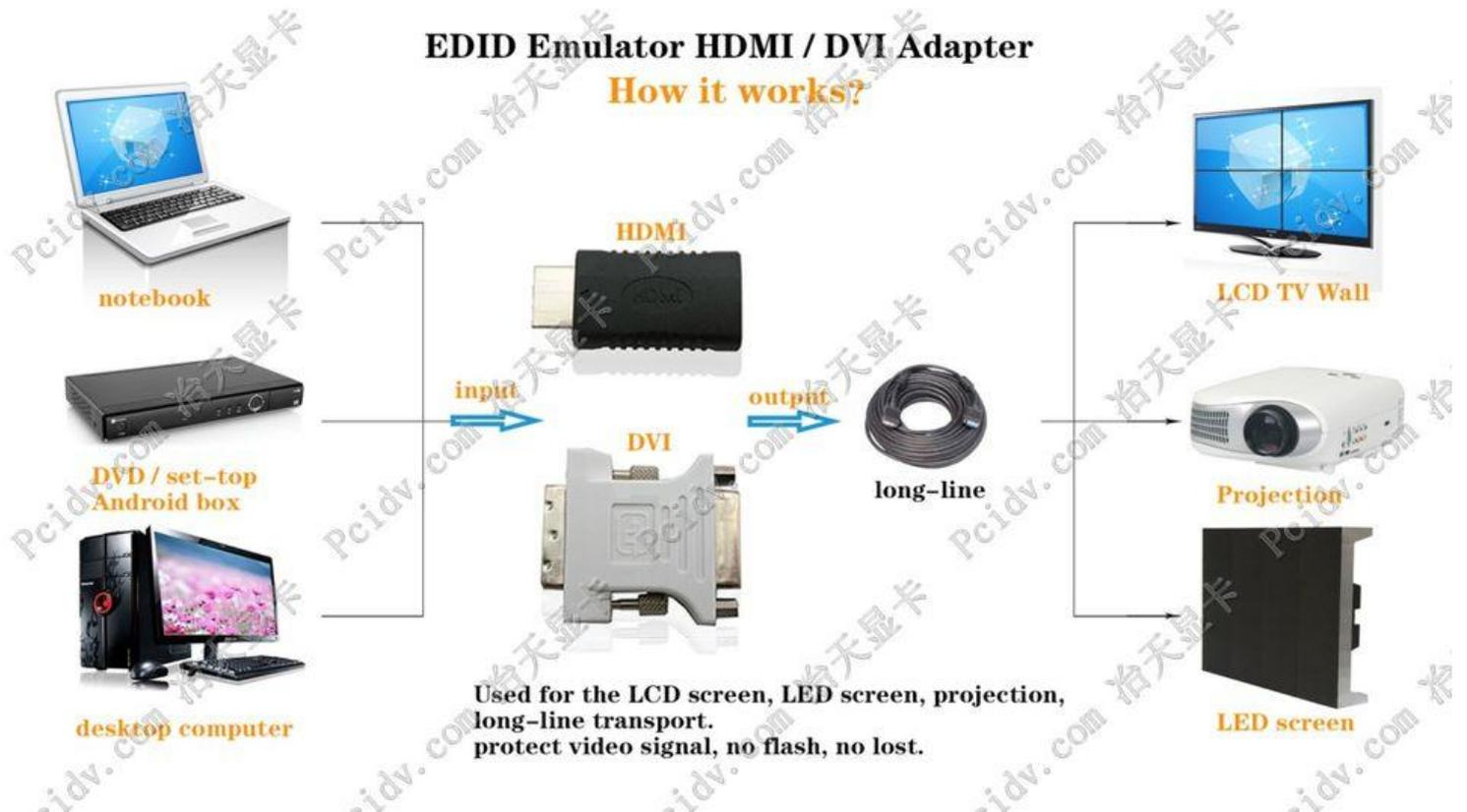
The EDID dongle is a simple to use DVI EDID Emulator, which is designed to emulate the EDID of a video display, providing constant and reliable EDID data to fix "Video Tearing Effect" for the a DVI source device and also support "No monitor display drop-out" for monitor disconnection or during power off for on-line display and video wall displaying avoiding Windows displaying configuration resetting.
